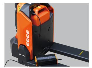
Socket on battery case for easy battery charging without necessity to take the battery out
